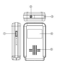
Power and Volume Switch Ear Phone Jack Probe Holder LCD Window Speaker
