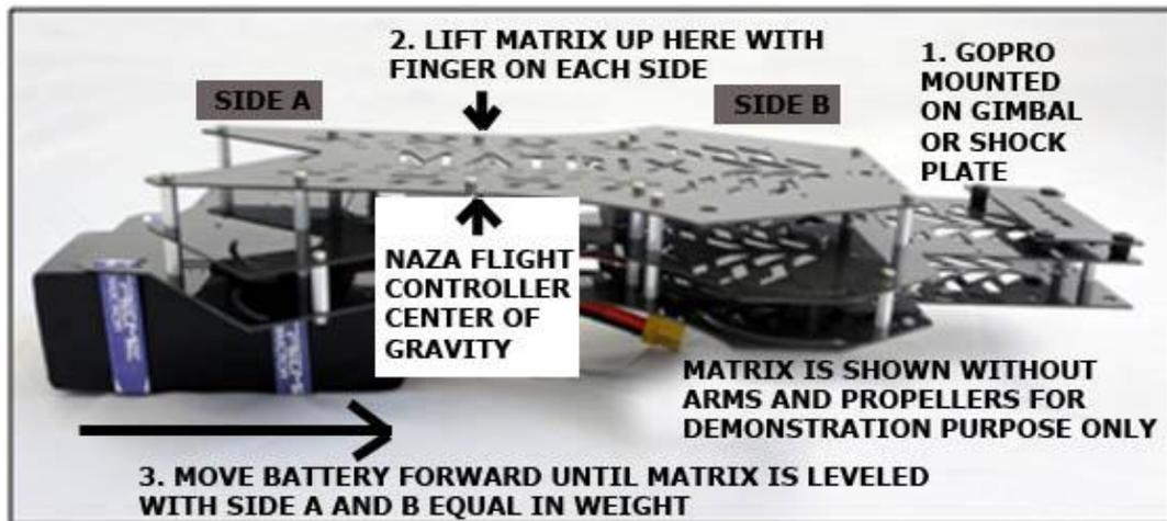
Figure 3.4-1 Balance at center of gravity
