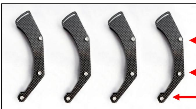
Figure 3.2-2 Four sets of Skid Landings assembled
