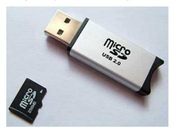
To avoid any plugging problem with a small connector and an easy-to-loose cable, we opted for a high-end flash memory card in the SD format (now microSD).
