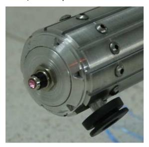
The Kill Key must be made out of a non-conductive material (PVC, Nylon etc).
