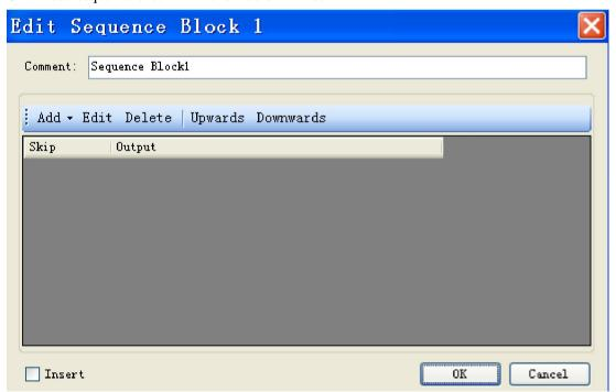
You can edit the program in this window. Upwards and downwards are used to change the position of the instruction in the block.
