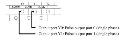
Below is the graph to show the output terminals and stepping driver wiring:
