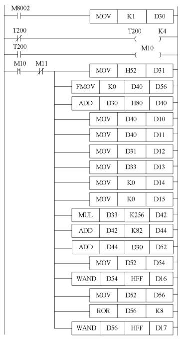
Write instrument's station Nr. K1 in to D30
