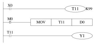
In the above example, MOV T11 D0, T11 represents word register; LD T11, T11 represents bit register.
