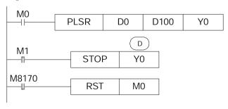
When M000 changes from OFF to be ON, PLSR output pulse at Y000. D0 specify the frequency, D001 specify the pulse number, D100 specify the acceleration/deceleration time; when the output pulse number reaches the set value, stop outputting the pulse; on the rising edge of M001, STOP instruction stops outputting the pulse at Y000;
