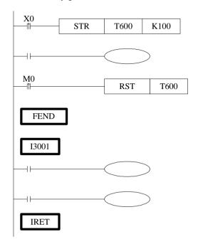
When X000 changes from OFF to be ON, timer T600 starts to time. When time accumulates to 100ms, set T600; meantime, generate an interruption, the program jumps to interruption tag I3001 and execute the subroutine.
