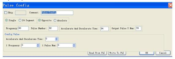
Set the pulse output frequency, numbers, output terminals, accelerate/decelerate time and so on. Then add the pulse instruction in the block:
