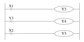
When executing dual output (use dual coil), the back side act in prior.
