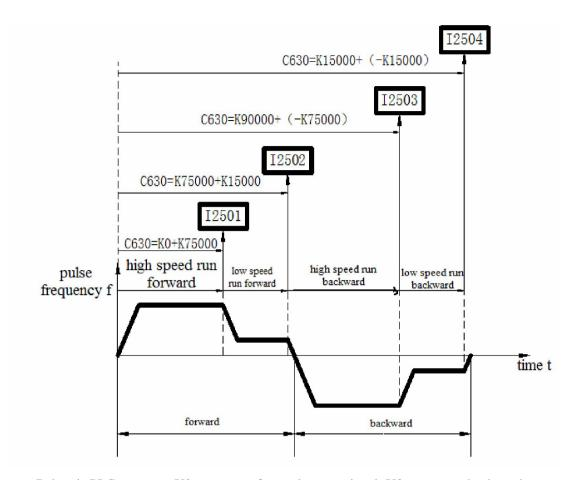
Below is PLC program: Y2 represents forward output signal; Y3 represents backward output signal; Y4 represents output signal of speed 1; C340: Back-forth times accumulation counter; C630: AB phase HSC;
