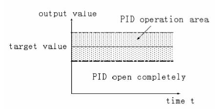
If the target value is 100, PID operation zone is 10, then the real PID's operation zone is from 90 to 110.
