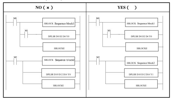
2. Do not use the same pulse output terminal in BLOCK and main program.
