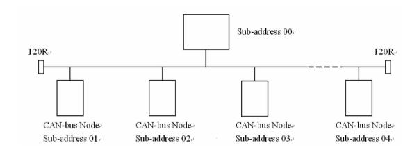
**CAN** (Controller Area Network) belongs to industrial area bus category. Compared with common communication bus, CAN bus data communication has performance of outstanding dependability, real time ability and flexibility.
