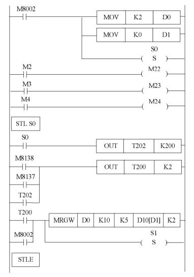
In PLC's first scan cycle, evaluate the "communication station" to be 2;
