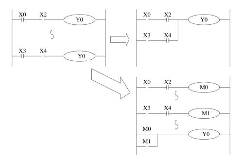
There are other methods. E.g. jump instructions or step ladder. However, when use step ladder, if the main program's output coil is programmed, then the disposal method is the same with dual coil, please note this.
