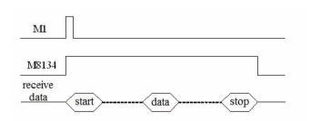
1: If you require PLC to receive but not send, or receive before send, you need to set the communication timeout as 0ms
