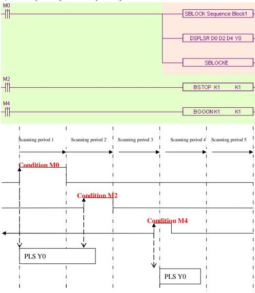
When M0 is from OFF ON, run "DSPLSR D0 D2 D4 Y0" in the BLOCK to output the pulse; when M2 is from OFF ON, stop running the BLOCK, the pulse will stop slowly with slope; when M4 is from OFF ON, output the rest pulses.
