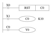
If cut the PLC power supply, the normal counter value become zero, the retentive counter can store the value, it can accumulate the value of last time.
