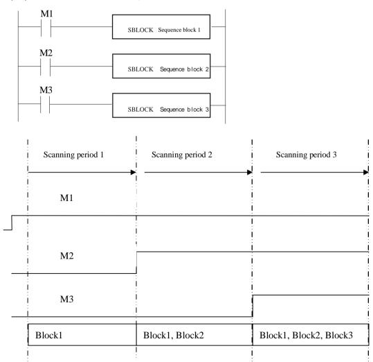
(B) the condition is rising or falling edge of pulse
