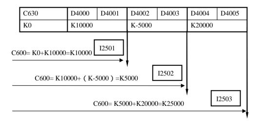
E.g. 2, the current value is C630 is 10000, the first preset value is 10000, the preset value in segment 2 is 5000, the preset value in segment 3 is 20000. When start to count, the counter's current value is 20000, generate first interruption I2501; When start to count, the counter's current value is 25000, generate first interruption I2502 ;When start to count, the counter's current value is 45000, generate first interruption I2503.
