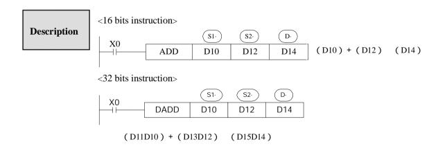
I The data contained within the two source devices are combined and total is stored in the specified
