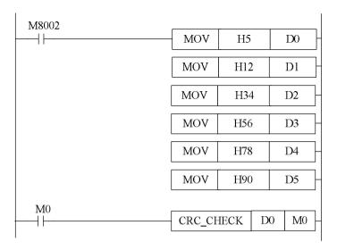
Download to PLC, then RUN PLC, set M0, via Free Monitor, we can find that values in D6 and D7 are the highest and lowest bit of CRC parity value;
