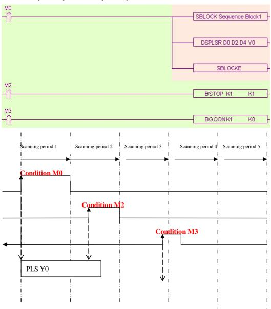
When M0 is from OFF ON, run "DSPLSR D0 D2 D4 Y0" in the BLOCK to output the pulse; when M2 is from OFF ON, stop the BLOCK, the pulse will stop slowly with slope, when M3 is from OFF ON, abandon the rest pulses.
