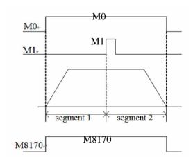
Take the sample program as the example, set two segments pulse output in D0, D1 and D2, D3, with the same frequency value; In second segment pulse output, set pulse number D3 as the output pulse number after receive M1 signal. This will realize "stop at certain length" function. See graph by the left side;
