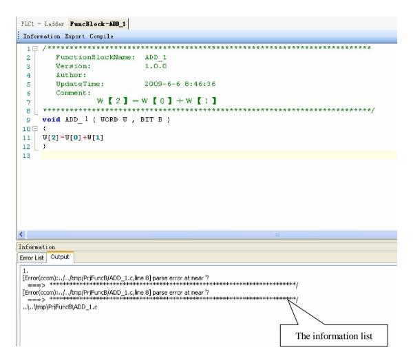
According to the information shown in the output blank, we can search and modify the grammar error in C language program. Here we can see that in the program there is no ";" sign behind W[2]=W[0]+W[1];
