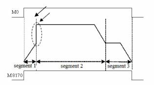
When outputting the segmented pulse, if the current segment's pulse has been set out, while meantime it doesn't reach the highest frequency, then from the current segment to the next pulse output segment, pulse jump appears, see graph above;
