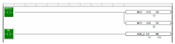
(5) From Free Monitor in he toolbar, we can see that D2 changes to be 30, it means the assignment is successful;
