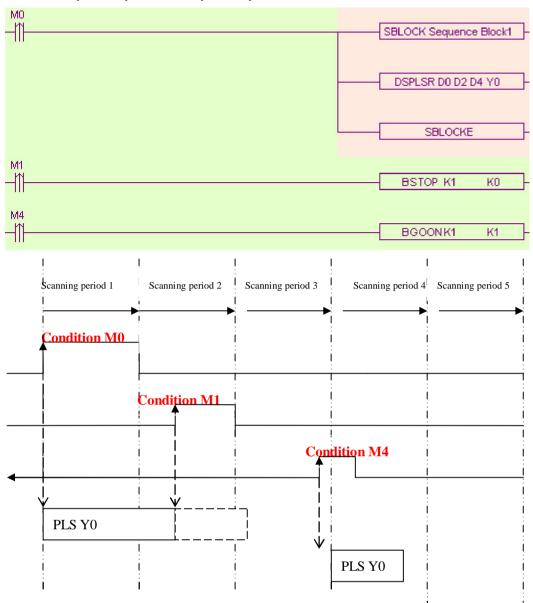
When M0 is from OFF ON, run "DSPLSR D0 D2 D4 Y0" in the BLOCK to output the pulse; when M1 is from OFF ON, the BLOCK stops running, the pulse outputting stops at once; when M4 is from OFF ON, output the rest pulses.
