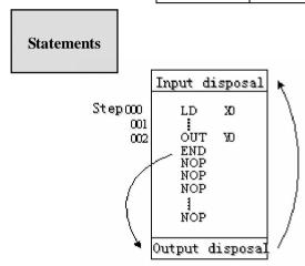
PLC repeatedly carry on input disposal, program executing and output disposal. If write END instruction at the end of the program, then the instructions behind END instruction won't be executed. If there's no END instruction in the program, the PLC executes the end step and then repeat executing the program from step 0.
