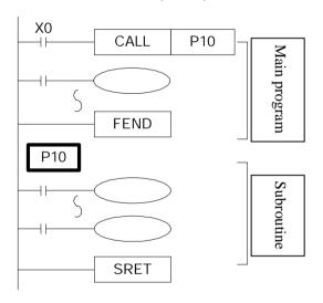
If X0 gets ON, jump to the subroutine from the main program; If the coil is not ON, run with the original program;
