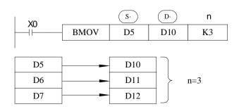
I As the following picture, when the data address overlapped, the instruction will do from 1 to 3.
