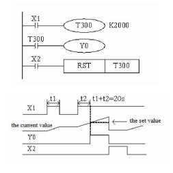
If X001 is ON, then T300 accumulate 10ms clock pulse based on the current value; when the accumulation value reaches the set value K2000, the timer's output contact activates. I.e. the output contact activates 2s later.
