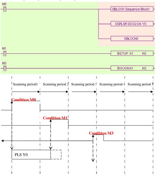
When M0 is from OFF ON, run "DSPLSR D0 D2 D4 Y0" in the BLOCK to output the pulse; when M1 is from OFF ON, the BLOCK stops running, pulse outputting stops at once; when M3 is from OFF ON, abandon the rest pulse.
