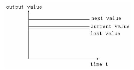
Suppose: we set the death region value to be 10. Then in the above graph, the difference is only 2 comparing the current value with the last value. It will not do PID control. The difference is 13 (more than death region 10) comparing the current value with the next value, this difference value is larger than control death region value, it will do the PID control with 135.
