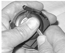
Fig. 125 - BATTERY HATCH REMOVAL (Tool)
