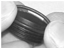
Fig. 131 - TRANSMITTER O-RING INSTALLATION
