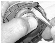
Fig. 130 - TIGHTENING VT3 HATCH RING
