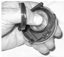
Fig. 129 - VT3 BATTERY INSTALLATION
