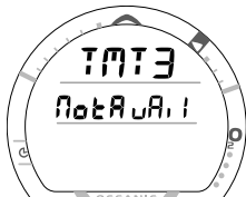
Fig. 6 - Transmitter 3 Status (Not Available)
