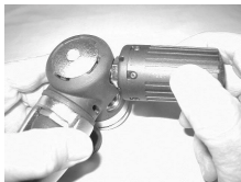
Fig. 134 -INSTALLING A TMT ON A REGULATOR
