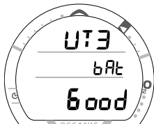
Fig. 4 - Battery Status (Good)
