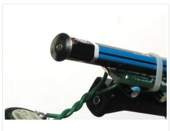
Next take 3 or 4" of copper tape and start wrapping around the bottom of the pencil, starting with the silver tab on the PCB and ending an inch before the end of the pencil. This will make contact with your hand and provide the second half of the sensor.
