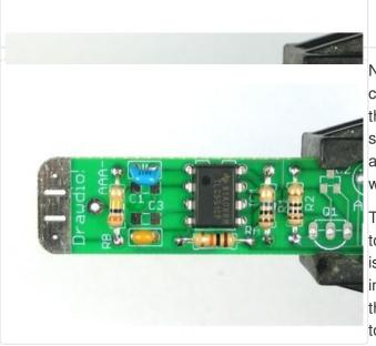
Next is the heart of the kit, a low voltage 555 timer chip. This one is called the TLC551. The important thing to note about the chip is that it is *not* symmetric. If it is put in wrong it will not work! Its also nearly impossible to fix if the chip goes in wrong so make triple-sure before you solder it in!
