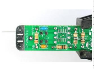
Next are the two ceramic capacitors **C1** and **C3**. Ceramic capacitors also have a nice property that they are symmetric/non-polarized. That means they can go in 'either way'. The capacitors are different values so make sure to not mix them up.
