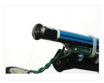
Next take 3 or 4" of copper tape and start wrapping around the bottom of the pencil, starting with the
