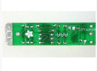
The electronic components are soldered in, next it is time to attach the speaker.
