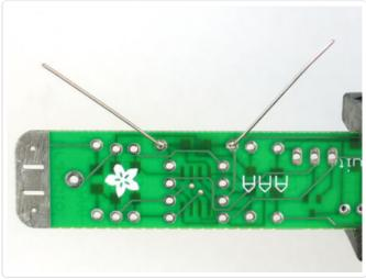
Place the resistor in the location marked **RA**.
