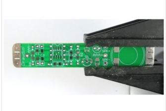
Get ready by placing the PCB in a vise.
