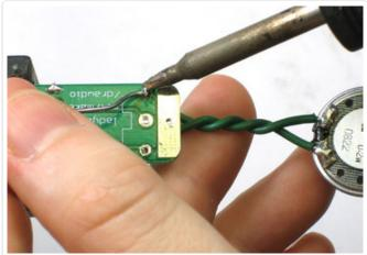
Solder the wires into place.
