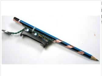
Finally, insert a battery into the kit. Then grip the pencil with one hand and touch the point of the pencil to your other hand. You will be able to hear the drawdio make noise!
