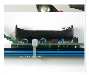
Next you can mount the PCB to your pencil. Place the PCB on the flat side of a pencil, and thread the zip tie through as shown and tighten it. You'll want it about an inch or less from the top of the pencil. The higher it is the more pencil you'll have to sharpen but it may be a little more unbalanced.
