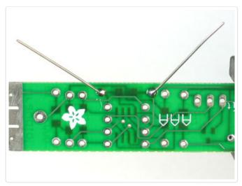
Using your diagonal cutters, cut off the long leads just above the solder joint.
