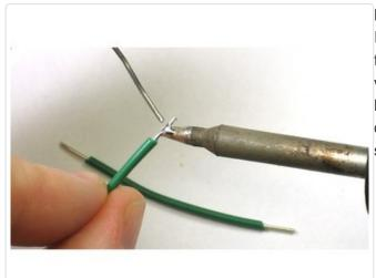
Next, it is a good idea to tin the ends of the wires. Its a little tricky because it requires holding three things. However, if you have a 'third hand tool' or a vise, you can use that to hold the wire while you heat up the stripped end and coat it with a little bit of solder. This will make it easier to connect to the speaker.
