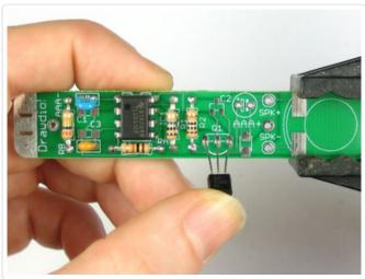
Next is the transistor amplifier **Q1** which is PNP type
