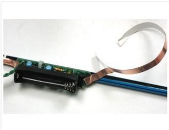
silver tab on the PCB and ending an inch before the end of the pencil. This will make contact with your hand and provide the second half of the sensor.
