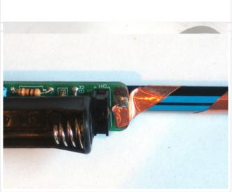
Solder the copper tape to the tab directly as shown.
