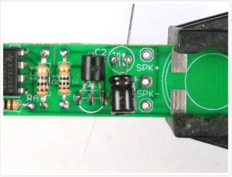
Fold the capacitor down so that it lies flat against the PCB.
