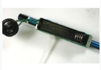
You can mount the drawdio to your pencil. Place the PCB on the flat side of a pencil, and thread the zip tie through as shown and tighten it. You'll want it about an inch or less from the top of the pencil. The higher it is the more pencil you'll have to sharpen but it may be a little more unbalanced.
