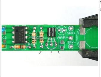
Now bend over the transistor so its 'face flat' against the PCB.
