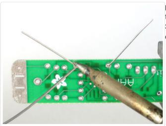
press and heat both the pad (the silver ring around the hole) and lead (wire) at the same time for 2 or 3 seconds. Then poke the end of the solder in to create a nice solder joint. Do this for both leads.
