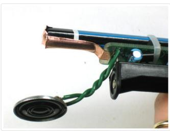
Wrap the tape along the top of the pencil so that the beginning is at the silver metal tab on the PCB, as shown.
