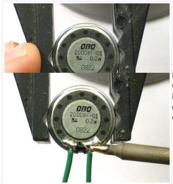
Next, warm up the tabs and slide the tinned ends of wire into the melted solder pool. Then remove the iron and wait a few seconds, the solder pool will cool with the wire in place. Do the same for the other pad.
