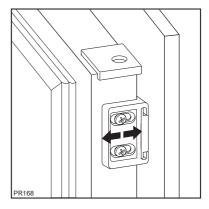
**9.** Should the lining up of the furniture door be necessary, use the clearance of slots. At the end of operations, it is necessary to check if the door of the furniture closes properly.
