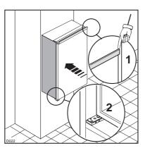
**1.** Push the appliance into the housing until stop strip touches the kitchen unit.
