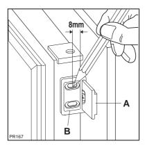
8. Open the appliance door and the furniture door at 90°. Insert the small square (B) into guide (A). Put together the appliance door and the furniture door and mark the holes as indicated in the figure. Remove the squares and drill holes with Ø 2 mm at 8 mm from the outer edge of the door. Place the small square on the guide again and fix it with the screws supplied.
