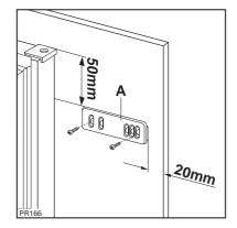
6. Place guide (A) on the inside part of the furniture door, up and down as shown in the figure and mark the position of external holes. After having drilled holes, fix the guide with the screws supplied.
