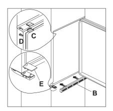
4. Snap vent gril (B) and hinge cover (E) into position.
