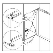
Open the door and push the appliance against the side of kitchen furniture opposite to that of appliance hinges. Fasten the appliance with 4 screws (I) provided in the kit included with the appliance.
