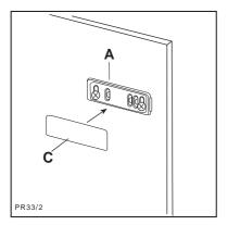
7. Fix cover (C) on guide (A) until it clips into place.
