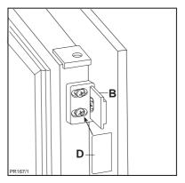
**10.** Fix cover (D) on guide (B) until it clips into place.
