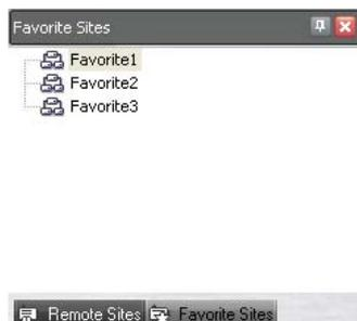
The **Favorite Sites** panel displays the list of Favorite sites registered during SISTORE AX RAS System setup. Selecting the Favorite site you want to connect to from the list and then dragging and dropping it on the screen connects all remote sites registered in the Favorite site automatically.
