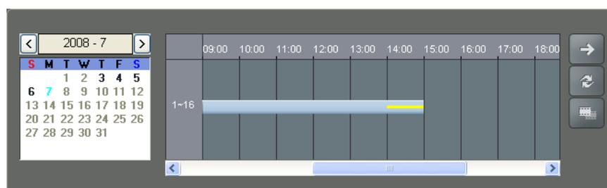
The recorded data of all camera channels are displayed by time in one-hour segments and a yellow-highlighted segment indicates the selected time that will be played back.
