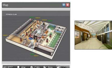
The **Map** panel pops up another screen when alarm-in, motion or video loss events are detected or when you click the device icon according to the **Map Editor** settings. Change the popup screen location by clicking the left mouse button on the screen and dragging it to where you want it located. Clicking the right mouse button on the popup screen displays the following popup menu.
