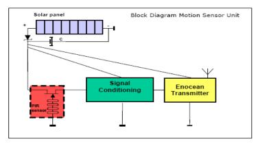
Fig. 4: Block Diagram
