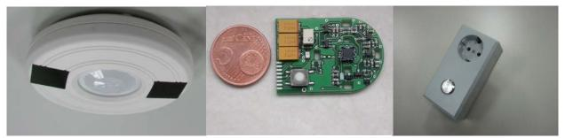
Fig. 1: Ambient light powered Motion Sensor
