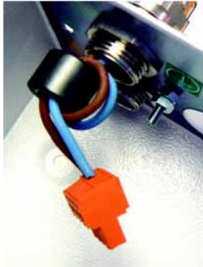
Figure 8: Looping relay connection wires around a suppression ferrite
