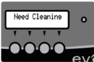
On the printer display, the message Need Cleaning appears. Cleaning is absolutely required after a print head change. No printing should be started before this operation has been completed.
