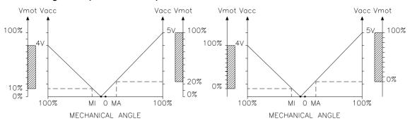
This function looks for and remembers the minimum and maximum potentiometer wiper voltage over the full mechanical range of the pedal. It enables compensation for non symmetry of the mechanical system between directions.
