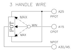
The Procedure for automatic potentiometer signal acquisition is carried out using the Hand Set. This enables adjustment of the minimum and maximum useful signal level, in either direction.
