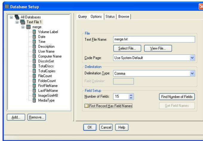
Figure 23: Removing Header Line
