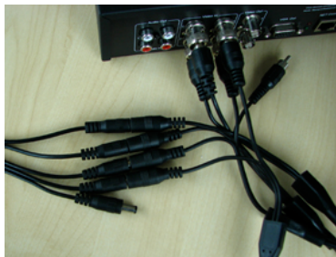
Example 4 channel DVR with camera cables plugged in
