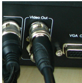
Example of a DVR with the BNC to RCA lead plugged in
