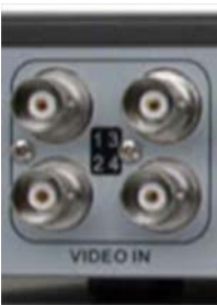
Example 4 channel DVR input sockets
