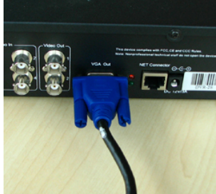
Example of a DVR with a VGA lead plugged in
