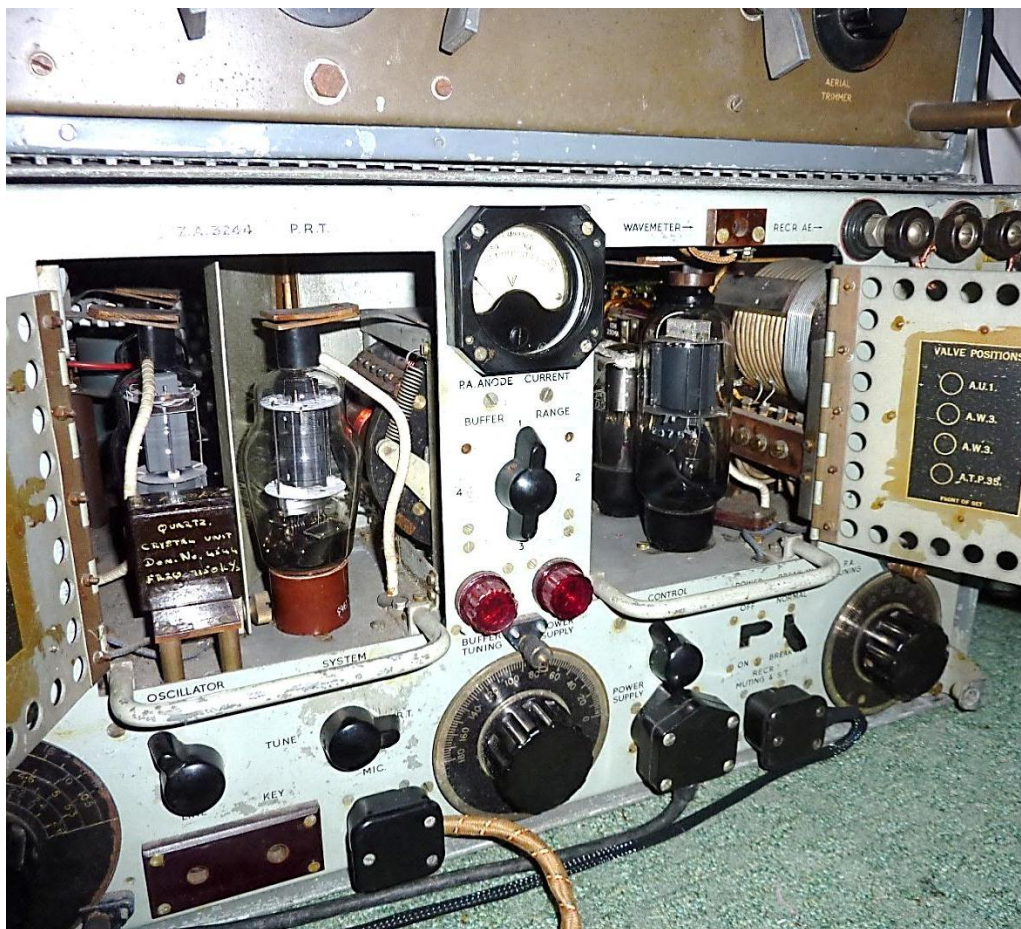
WS12 (part of a quite rare WS12/R107 combination dating from 1941 and pictured on the back page of the current Issue of Signal) belonging to Mike Buckley M1CCF, being restored by Martin Smyth M0MGA
