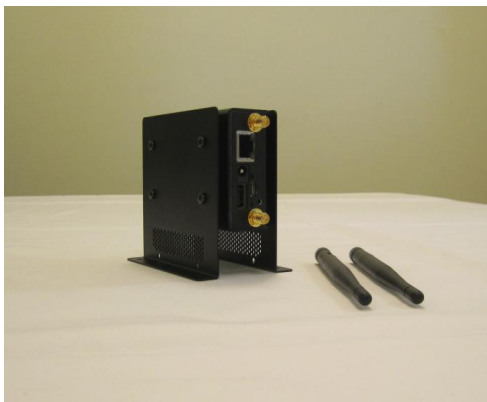
Figure 11. M2M System with 2x 802.11/802.15.4 antennas
