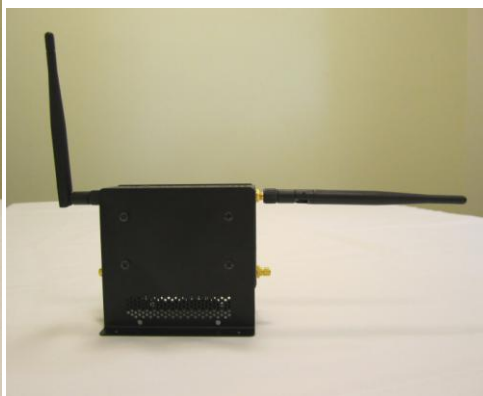
Figure 12. M2M system with 2x 802.11/802.15.4 antennas installed
