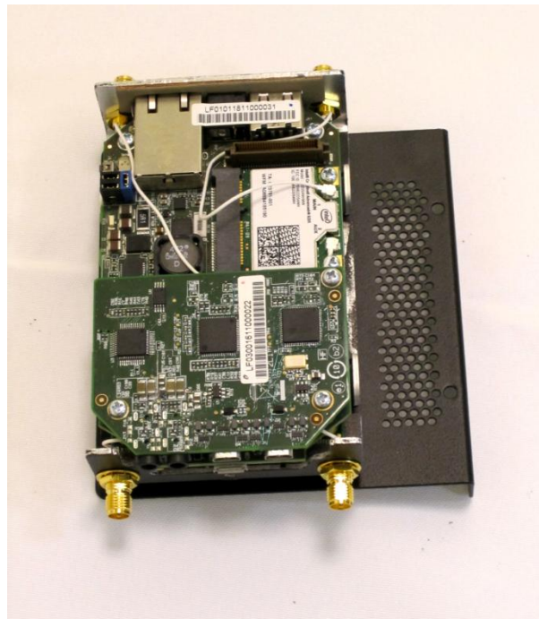
Figure 32. The M2M System with the 3G module fully installed
