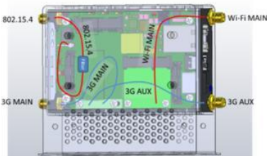
Figure 24. Antenna Cable Routing supporting 3G Usage
