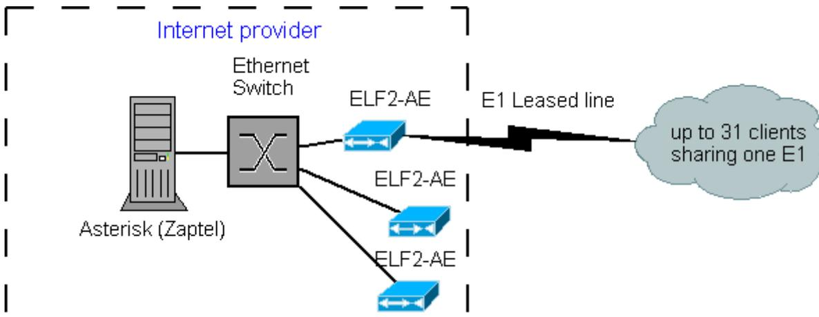
The ELF2-AE device and software **DAHDI** package allow to create [reasonably priced platform](#) for providing clients with separate data transmission channels.
