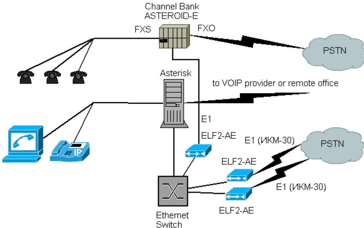
In this scheme the office can be connected to the IP telephony provider or corporate VOIP network, telephony costs decreasing.
