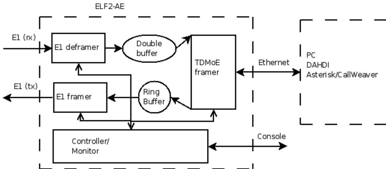
**Figure 1. Internal ELF2-AE architecture**
