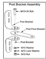
2. Attach the Post Bracket Assembly and the Gate Bracket to the gate opener with the clevis pins. Secure the clevis pins with the hairpin clips
