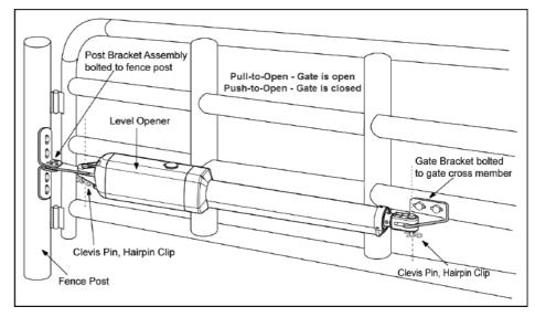
13. Open the release hole plug on the top of the gate opener, insert the release key, and turn the key 90° counterclockwise. This restores normal operation.
