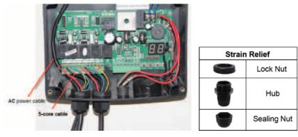
2. Connect the AC power supply cable to the control box as shown in the following illustration:
