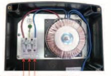
Terminals for the power supply. Connect the Live Line and Null Line to the "L" and "N" terminals respectively. Connect the GROUD wire to the "GR" terminal.
