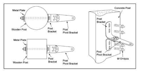
CAUTION: Ensure the post or wall the gate opener bracket will attach to is large enough to handle the load of the gate. This post will be under constant stress when opening and closing. Do not attach the bracket to a weak or unsteady post.
