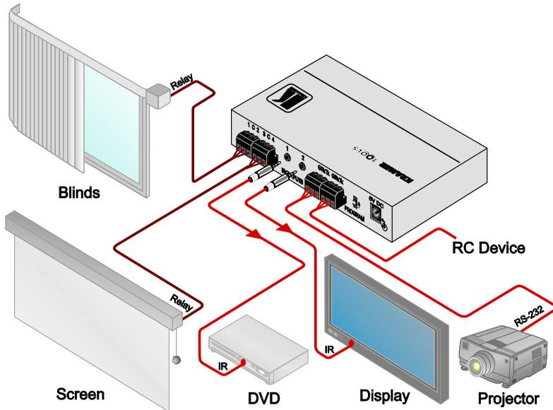
Figure 2: Connecting the PL-18 Control Port Expander
