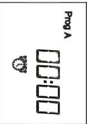
You can start a watering cycle up to 8 times per day and per program if you prefer short watering cycles. Select the desired program by pressing the key to set the first start time; Use the and keys to set the first start time. Then press the key to move to the next start time.
