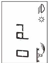
You can delay watering from 1 to 15 days during rainy weather.
