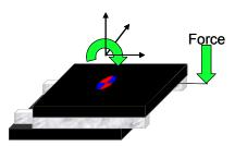
Given a MX80L-T02 with a 2 kg load mounted 35 mm off of the end of the carriage in line with the travel path. The lever arm is 35 mm + 40 mm (center of table to edge) = 75 mm
