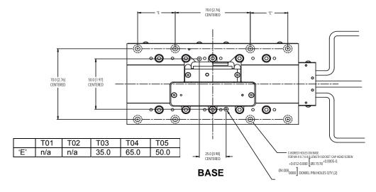
The positioner must be mounted to a flat, stable surface, with a flatness error less than or equal to 0.025mm/300mm for operation (specifications will be greatly varied from published specification).
