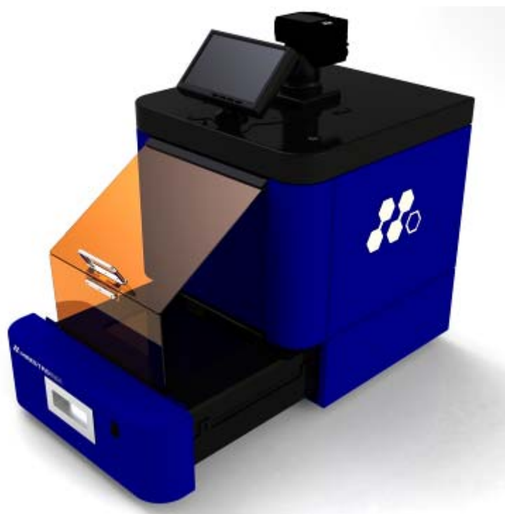
LED transilluminator pulled-out for gel cutting with amber filter
