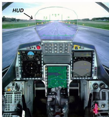
Figure 1: Position of the Head-Up Display in the cockpit of JAS 39 Gripen
