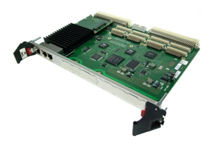
The A21C is a Freescale<sup>™</sup> QorlQ<sup>™</sup> based single-board computer for embedded industrial applications. The SBC features full VME64 support and can be used as a master or a slave in a VMEbus environment. The A21C provides 1 MB local dual-ported SRAM for slave access and communication between the local CPU and another VMEbus master.
