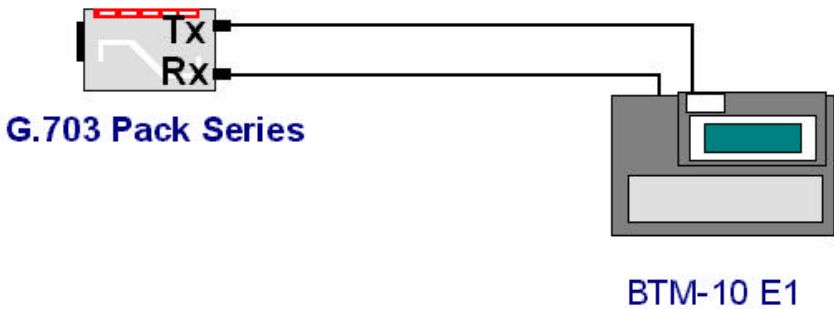
Figure 3-1: Test setup, E1 link
