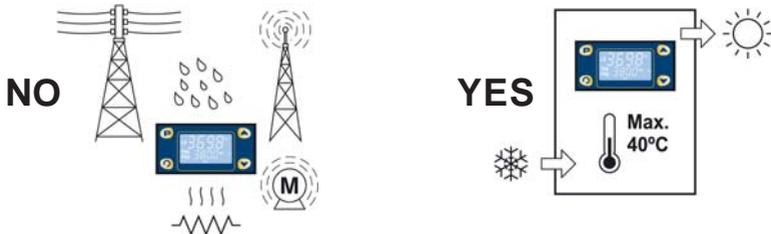
The connections must be done separating, phisically, the measurement signals from the control or power signals.
