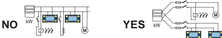
In a general way, it is recommended to use an exclusive supply line for the equipments connected directly from the main and provided with the appropriate protections. If this is not possible, install an isolation transformer with the shield connected to ground.
