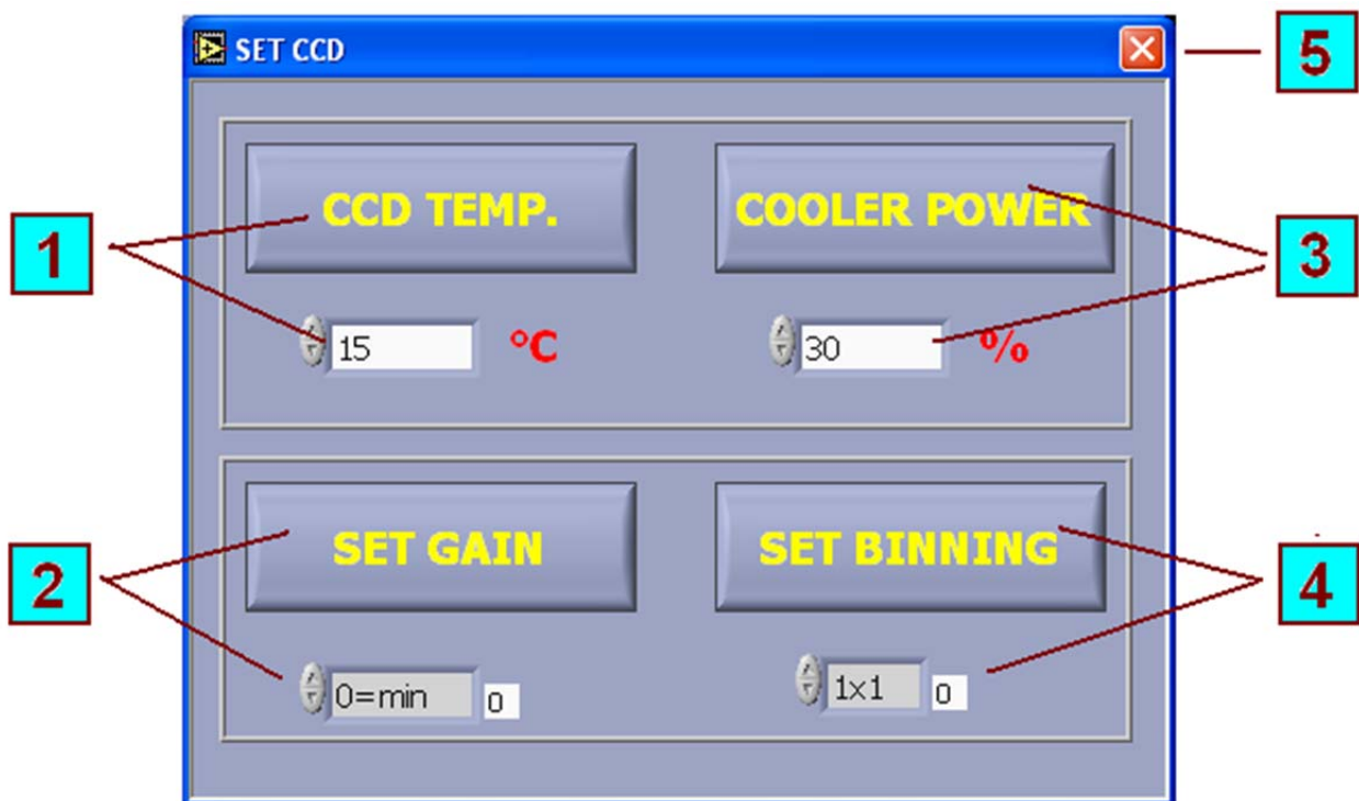
Figure 3 – The SetCamera.vi panel. It allows one to set the camera working mode.
