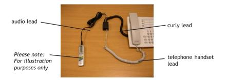
OPTION 2 - Line recording (using telephone lead)
