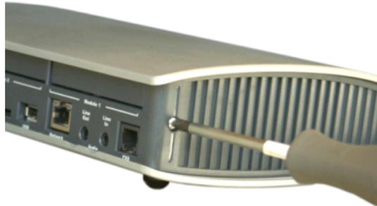
Remove the top cover. You must be grounded with an anti-static wrist strap. Plug in the end of the serial cable provided with the appliance to the connector as shown below. The cable can only be plugged in to the connector using the correct orientation. Connect the other end to the serial port on your development computer.
