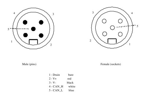
Figure 4-3 DeviceNet Connectors
