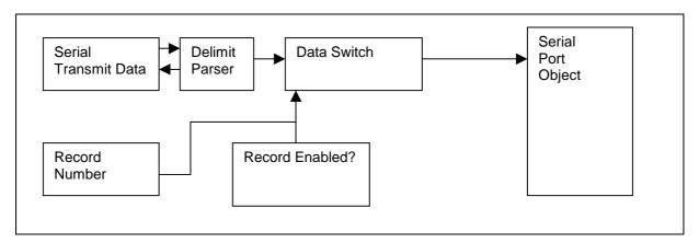
Figure 7-1 Transmit Record Algorithm Functional Flowchart
