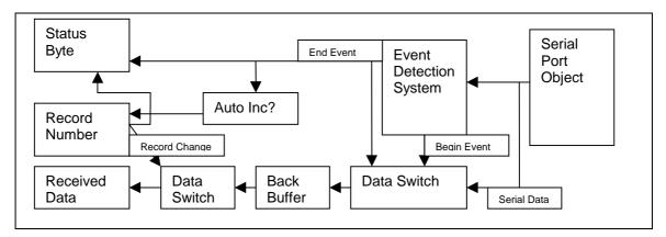
Figure 7-2 Receive Record Algorithm Functional Flowchart
