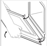
**4.** Put the door on a soft cloth on a stable surface.
