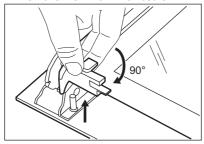
First lift carefully and then remove the glass panels one by one. Start from the top panel.
