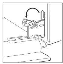
Close the oven door halfway to the first opening position. Then pull forward and remove the door from its seat.
