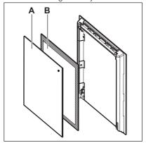
Make sure that you install the middle panel of glass in the seats correctly.
