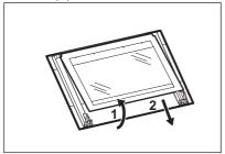
8. Clean the glass panels with water and soap. Dry the glass panels carefully. When the cleaning is completed, install the glass panels and the oven door. Do the above steps in the opposite sequence.
