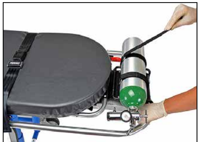
Figure 23 - Securing the Oxygen Bottle
