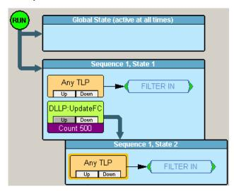
**Result**: Only TLP (any type) is in the CATC Trace. **Reason:** In both states, the rule is to keep only TLP.
