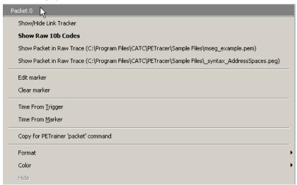
Step 2 Choose Edit Marker and enter a new identifier into the Edit Marker for Packer # pop-up, or Choose Clear Marker. When you choose Clear Marker, the marker is removed and the red line disappears.
