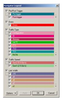
The Navigator Legend dialog box has areas corresponding to each of the panes. Each area has check boxes that allow you to hide/display information in the pane. You can set the priority of information displayed in the panes using the up and down triangles on the right.
