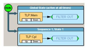
Result: TLP:Completion and TLP:Memory are filtered out.
