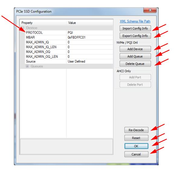
All the fields in this dialog are required and editable. Make sure that the information entered is correct. Click on any field and the description displays in the bottom read-only box (see figure on page 231). Some important fields are described below:
