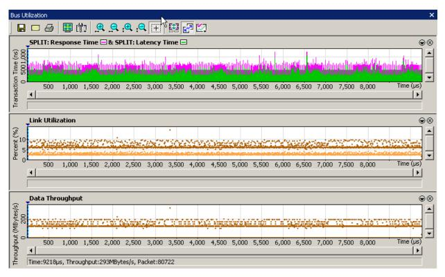
The Bus Utilization window displays information on bandwidth use for the transmit and receive channels.
