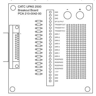
The Breakout Board connects via a cable to the **Data In/Out** connector located on the rear of the Analyzer unit. Each signaling pin is isolated by a 100  $\Omega$  series resistor and a buffer inside the Analyzer unit.
