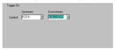
By default, these selections include standard K (command) characters for each direction (upstream and downstream). You may also manually enter a D (data) character in the upstream or downstream boxes.
