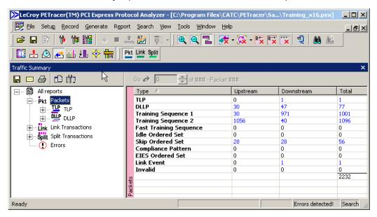
Step 2 Click the up or down arrows of . The CATC Trace jumps forward or backward through the display to the next instance of selected protocol level.
