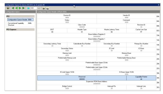
Select **Show Configuration Space for xxxx** from the menu, where **xxxx** is the device number. The Configuration Space View opens.
