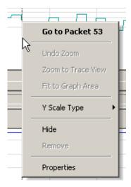
Go to Packet #: Relocates the CATC Trace to the selected packet number.
