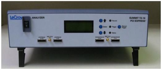
With advanced features such as support for PCI Express Spec 2.1, data rates of both 2.5 and 5 GBps, lane widths from x1 to x16, and a full 8 GB of trace (recording) memory, the Summit T2-16 provides unmatched capability and flexibility for developers and users of advanced PCI Express products. The Summit T2-16 is the most advanced and sophisticated PCI Express Analyzer available in the market today.
