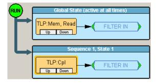
Result: Only TLP:Completion and TLP:Memory are in the CATC Trace.
