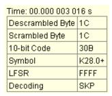
**Note**: Descrambled values can only be displayed after the first recorded skip ordered set. Data prior to the skip is displayed in scrambled values, due to the unknown LFSR.
