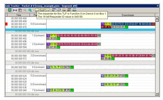
Each time slot in the vertical axis represents the minimum time that a DWORD requires to traverse the bus.
