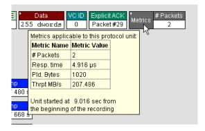
**Note:** The tool tip also presents information for time passed from the start of the recording till the beginning of this Link or Split Transaction.
