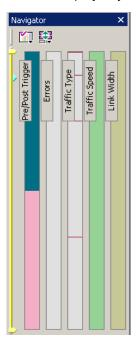
From left to right, the panes are: Pre/Post Trigger, Errors, Traffic Type, Traffic Speed, and Link Width. Each pane represents the entire CATC Trace with respect to different types of information. The top of each pane represents the start of the CATC Trace file, and the bottom represents the end of the CATC Trace file.
