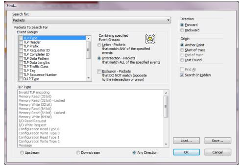
**Step 3** From the Search For menu, select a display level such as **Packets**. To search multiple levels, finish steps 3 to 9, and then repeat 3 to 9 for each additional display level.
