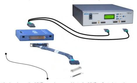
Connect the header on the MidBus probe assembly to the MidBus footprint on the System Under Test (host platform/root complex). The following picture shows two midbus footprints, with one connected to the MidBus probe assembly:
