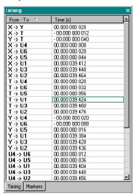
Timing measurements between all combinations of X, Y, U, and Trigger cursors are in the Timing window.
