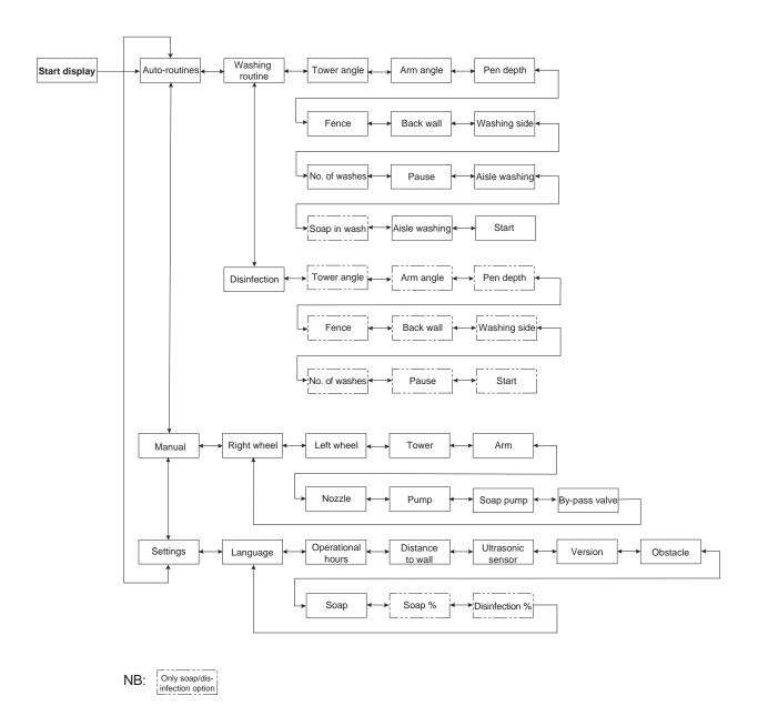
By means of the arrows the user can get around in the menu system. When the MULTICLEANER has been connected to the power supply, it will be ready for operation after 30 sec. Then the display will show a start-up screen, on which the user will be asked to press arrow the right to initiate the MULTICLEANER.
