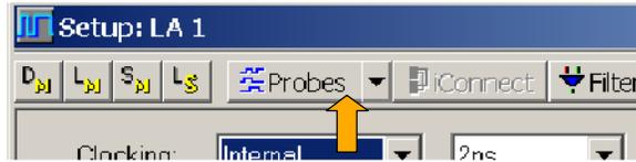
The Probe Properties dialog box opens showing the probe activity. When the target system is off, or no probes are connected, there is no probe activity. The channels are shown as active low signals.
