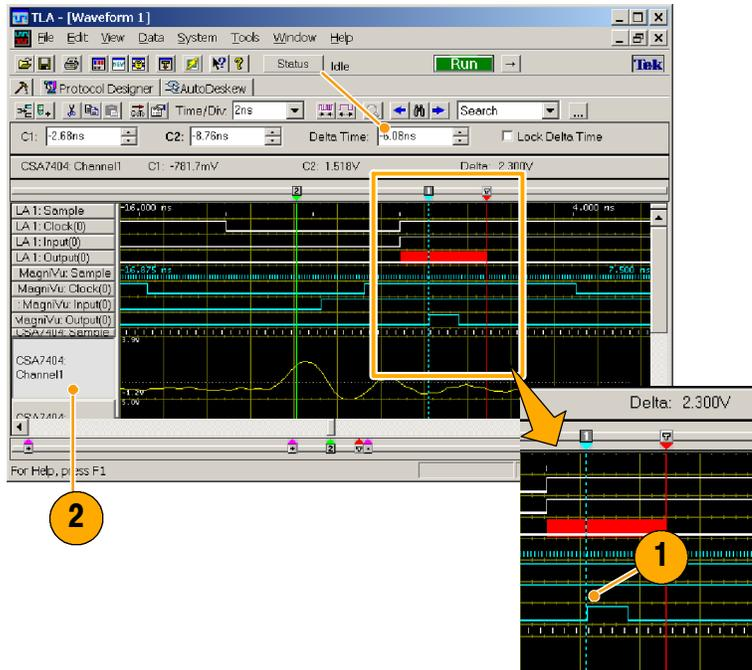
3. Move Cursor 2 to the point on the glitch where the waveform crosses the threshold voltage as indicated by the measurement readout.
