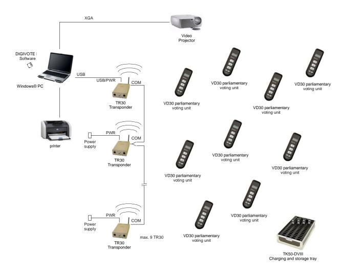
This configuration allows a total distance about 1000 meters. The "inner" transponders are connected by means of special adapters. If required our planning department will assist you.
