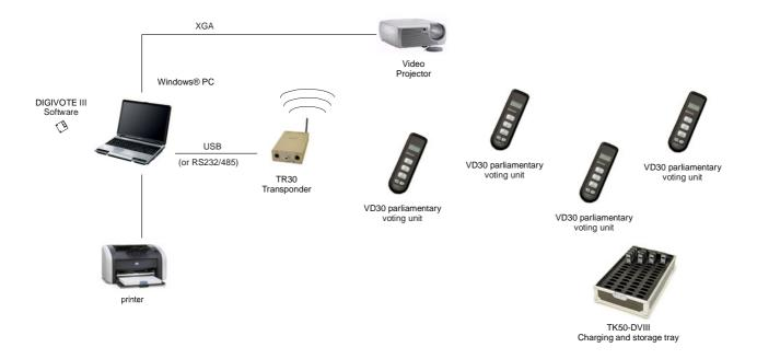
The working range between the transponder and the voting unit is up to 50m (radius), depending upon the specific location and the building conditions.
