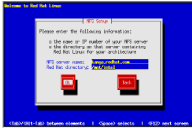
Figure 3.11: Installing via NFS
