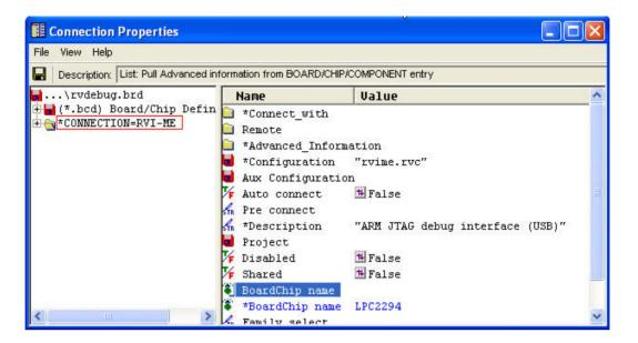
After the configuration, you can close the "Connection Properties" window, shown above, and confirm to save the configuration.
