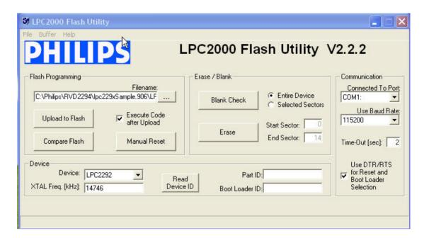
Just use the setting above and make sure "Use DTR/RTS for Reset and Boot Loader Selection" is checked. The YL-LPC2294 Development Board BIOS sample image can be found under
