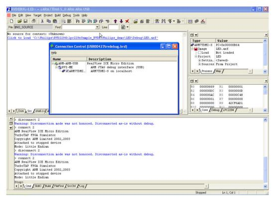
Clicking hyper link "...\Debug\LED.axf" as seen above will load the LED sample image onto the internal SRAM of LPC2294 for execution. Clicking "Debug", "Toggle Source/Disassembly", the source window will show mixed code. At address 0x4000 0000, the first instruction is "Reset LDR PC, ResetAddr", indicating the image has been loaded onto the internal SRAM area successfully.
