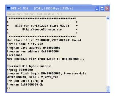
4) Change the jumper setting, close JP1 jumper 2+3 (EXTRE\_BOOT) to external reboot, then press the red reset button. After reset, the system will boot from external Flash, and the LED example will result in LEDs D1~D8 on the Development Board blinking on and off in a circular fashion at equal intervals.
