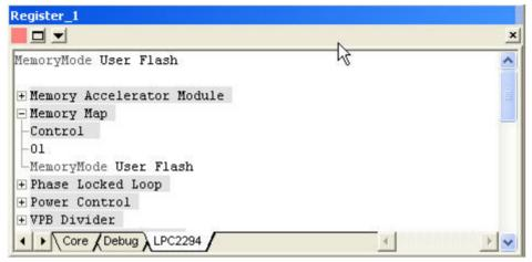
Go to "Memory Map" and make sure "Memory Mode" is set to 0x01 or "User Flash". This is to ensure Memory Map Control register is set to "User Flash Mode", and interrupt vectors are not remapped and reside in internal flash. For more details, please refer to System Control Block chapter, "LPC229x User Manual".
