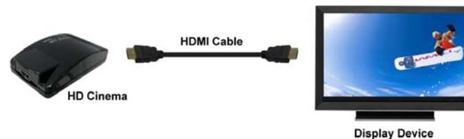
**NOTE:** You can also use a HDMI to DVI cable to connect between the HD Cinema and your display device (the display device must have a DVI input).
