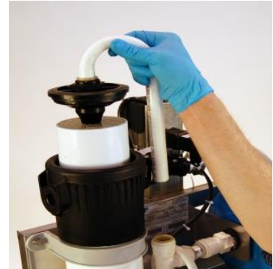
Figure 7.3: Lifting top hatch and filter element
