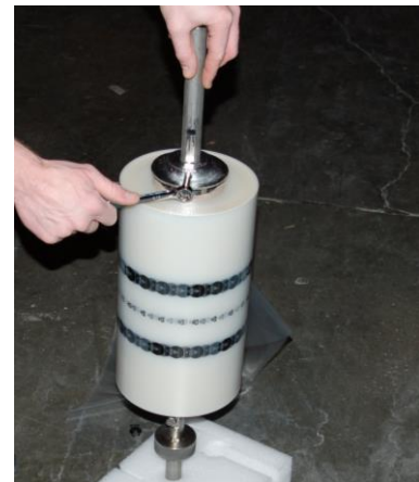
Figure 8: Removing left cone from Shaft
