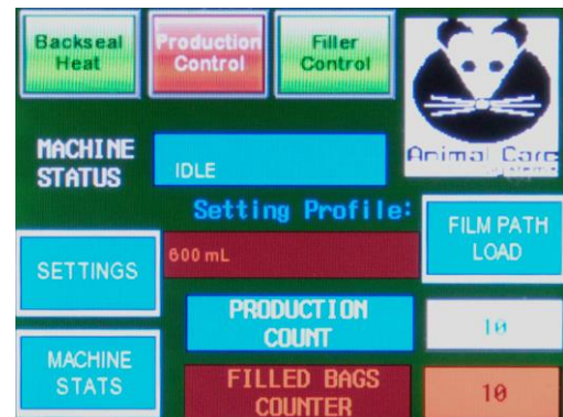
Figure 4: Home Screen; (Production Control shown in Off position)
