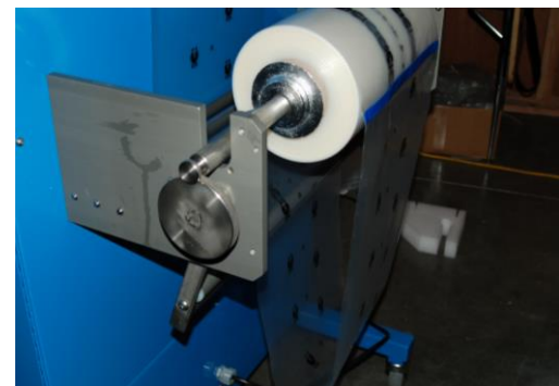
Figure 9: Film feeding from rear of roll to Tension Bar
