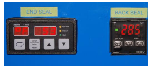
Figure 5: Sealer Heat Controls Green light indicating Backsealer fully heated
