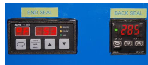
Figure 4.3: Sealer Heat Controls; Green light indicating Backsealer fully heated
