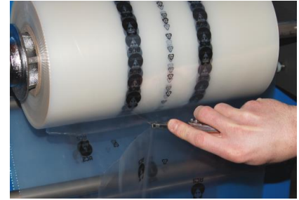
Figure 6.3: Cutting film from roll
