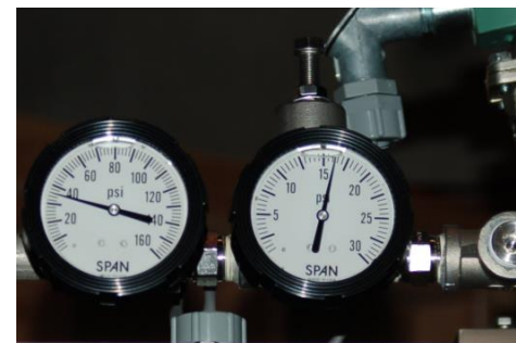
Figure 4.2: Input (Left) and Regulated (Right) Pressure Gauges
