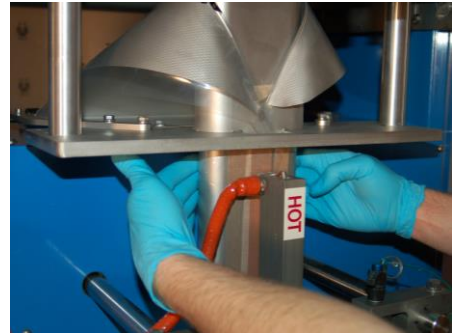
Figure 6.12: Guiding film downward along Forming Channel
