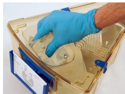
Figure 4.11: Pressing bag into cavity, bag pierced
