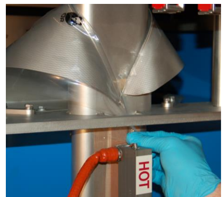
Figure 6.11: Film pulled through Base Plate
