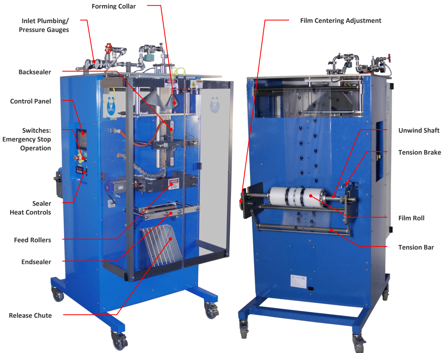
Figure 1: Primary Optiquench components
