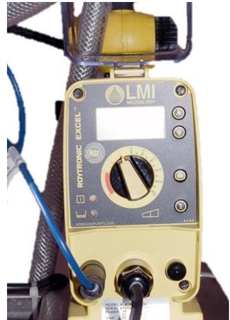
Figure 5.4: Dosing Pump; Buttons along right side (top to bottom): Up/Down, Mode, Power
