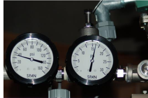
Figure 3: Input (Left) and Regulated (Right) Pressure Gauges
