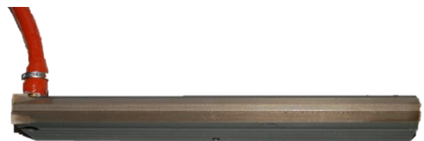
Figure 6.23: Fresh tape applied to seal bar
