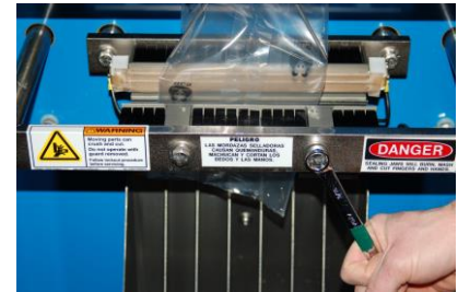
Figure 6.17: Removing unheated side of Endsealer
