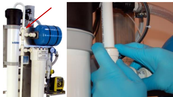
Figure 7.2: Locking sleeve depressed
