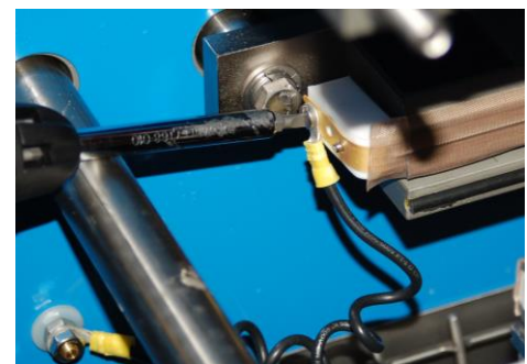
Figure 6.19: Dismounting cut wire from spring-loaded mounting block
