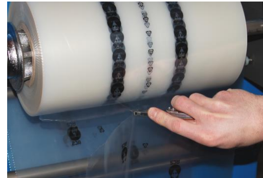
Figure 6: Cutting film from roll
