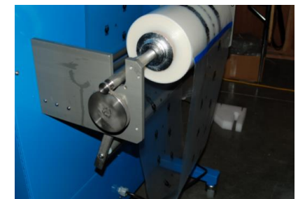
Figure 6.7: Film feeding from rear of roll to Tension Bar
