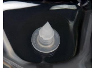
Figure 4.9: Valve installed in water bag holder
