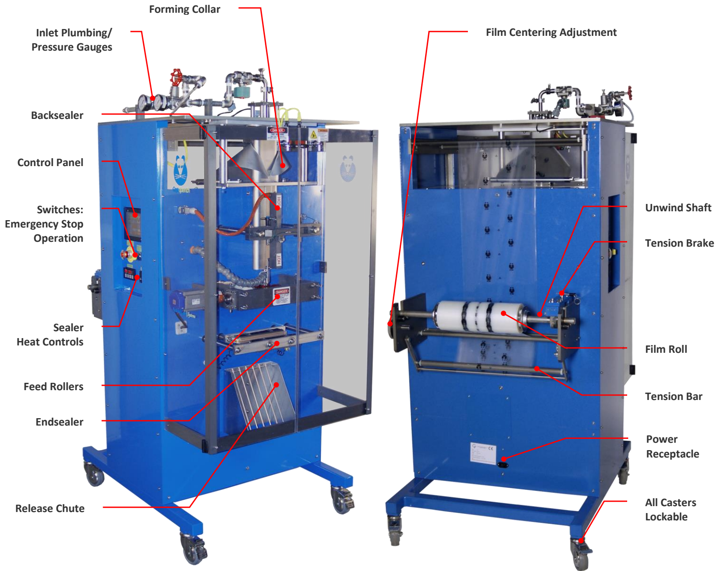
Figure 3.1: Optiquench Bag Filler primary components
