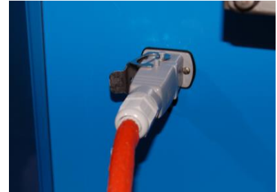
Figure 6.20: Backsealer electrical connector with locking clip unlatched
