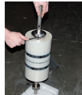
Figure 6.5: Removing left cone from Shaft
