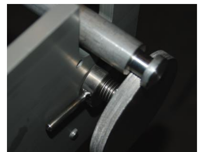
Figure 6.2: Film positioning wheel and specialized jam nut
