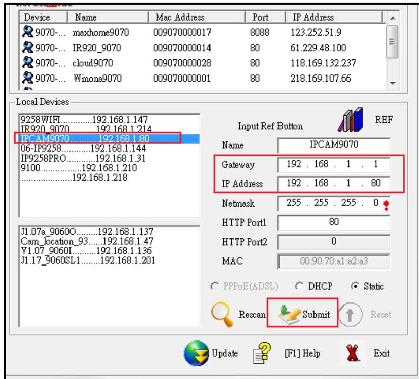
4.) Then hit the rescan button on IP Edit to confirm the changes have been made.
