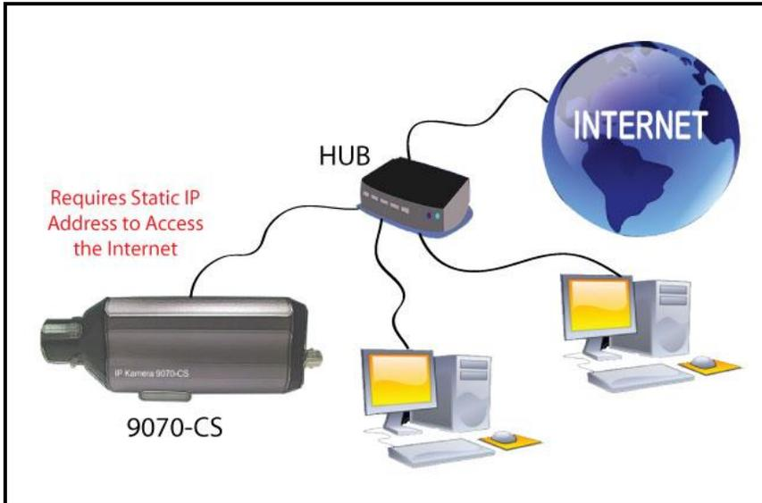
In this case, the 9070-IR is being connected to the internet through a hub, which is different from a router. The hub does not provide DHCP, and therefore would require that this setup have a static IP Address that is provided by the ISP.
