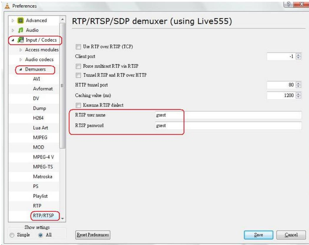
6.) Check the Cache value. *For low latency, it should be 70~80 based on PC's performance.*
