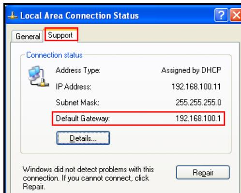
**IP Address:** Make sure the first 3 sections of the IP Address matches the gateway address.
