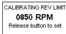
As the engine is revved, the RPM speed will alter on the display. Once the desired launch rev limit has been reached, release the selector button – the new rev limit will now be set.
