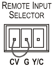
Figure 7: Connecting the Contact Closure Remote Control PINs
