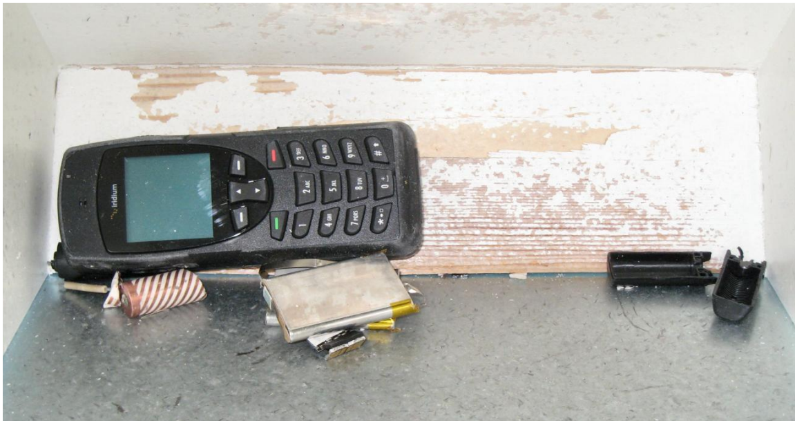
Figure A-1. Iridium 9555 Phone after 1 meter random drop tests
