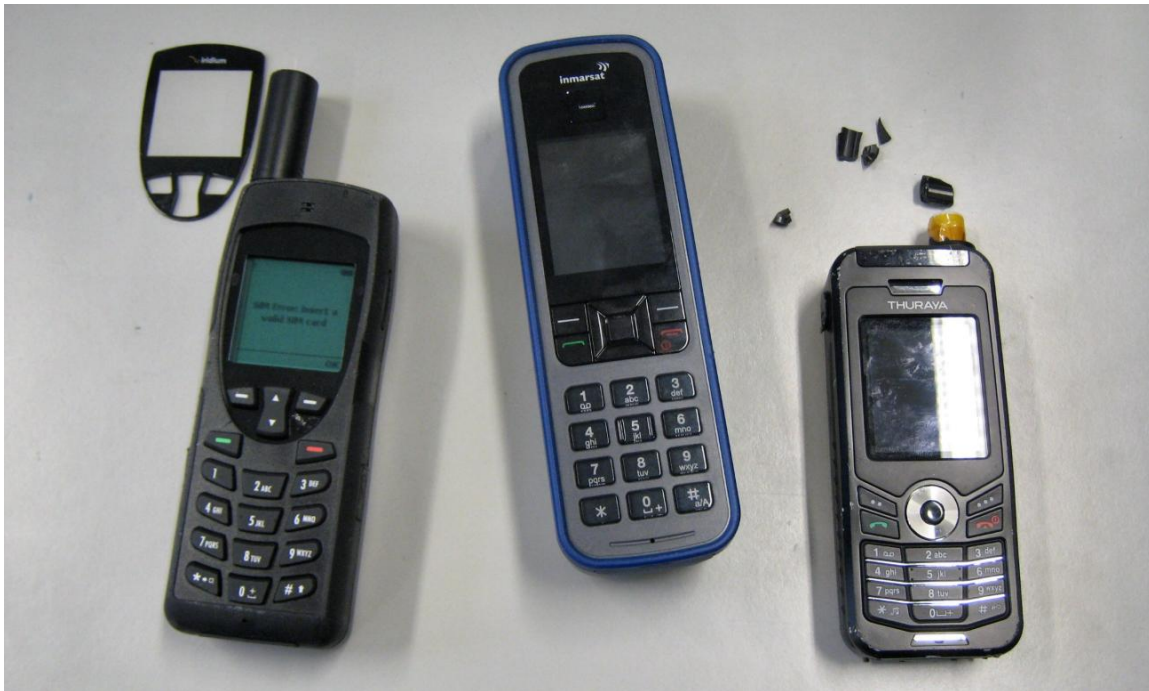
Figure A-2 Satphones after 1, 1.5, and 2 meter guided freefall tests
