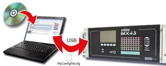
Figure 1: The COM43 application allows MX43 configuration on a PC as well as bidirectional transfer of the configuration file via USB
