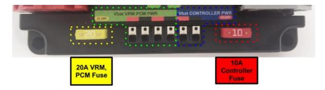
Both automotive fuses are type **ATM** automotive blade mini fuses. Spares can be purchased at most hardware stores (Do **not** purchase ATC as they will not fit).
