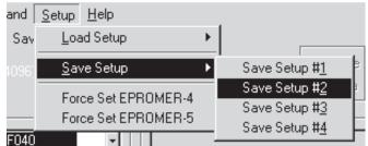
When you click any of those options, used or empty, it will appear a text input screen, asking you to name this setup. You can enter any name you want, with spaces or not, is up to you to identify this special setup of the Epromer.
