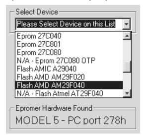
If you select a device that could require programming voltage different from the regular 12.5V, such as 2732 eprom devices, a selection for 21 and 25V will be enable, so you could select the proper programming voltage for that device, as shown below;
