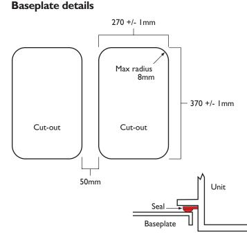
If the cartridges need to be secured in position the top edge of the base flange can be used to clamp against. Care should be exercised to ensure the base seal is not distorted to the point it fails to seal if the cartridges are fastened or clamped in position. The outside edge of the upper surface can be used to seal against if the cartridges are to be used in a fully ducted system.
