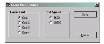
Once selected, a dialog box requesting the user to select a "Comm Port" and "Baud Rate" will be displayed. The default setting is COM1 at 9600 baud.
