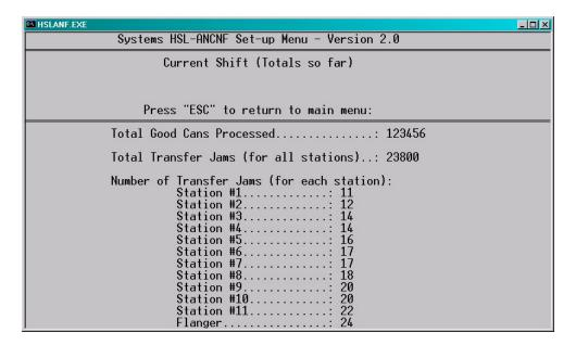
This data is the totals so far into the shift. This data is transferred to the "Last shift" data when the end of shift input transfers from a "0" to a "1". This can be at the end of either an 8 or 12 hour shift or alternatively could be done at label changes such that the data collected would be for label runs rather than complete shifts. This data cannot be reset either from this menu or by the operator, only at the end of shift input transition. To exit back to the main menu, press <ESC>.
