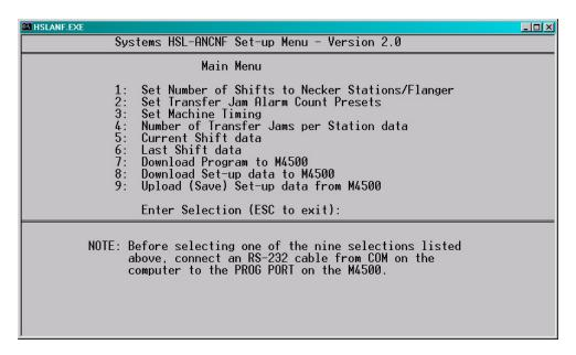
**Note:** The "HSLANCNF" program is an on-line communications program used to interface with the M4500 module. The data displayed in the menus and set in the menus is communicated directly to the M4500. Therefore, prior to selecting any of the above selections, make sure an RS-232 cable is connected from the COM port on the computer running "HSLANCNF" to the "PROG" port on the M4500.
