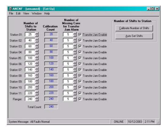
**Number of Shifts (Stations 1 thru 10 and Flanger):** This is the number of shifts from the infeed screw sensor to the transfer sensor for each station. These numbers can be determined using the calibration mode or they could be counted manually if desired. The range of values for these numbers is 1 to 319. In addition, the transfer jam detection can be disabled by setting the "number of shifts" for the respective station to "0". This would be done on machines not equipped with all stations.
