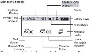
The pager returns to the standby screen after the time out period. Time, date, battery level and Private Time are displayed in the standby screen. Press any button to return to the Main Menu Screen.
